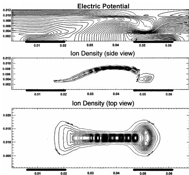
Figure 5. Equipotential lines, and the ion density ("top" and "side" views) after the beginning of the discharge (330ns) for the case of  $V_{addr}=10V$  ( $V_{ON}=60V$ ).
