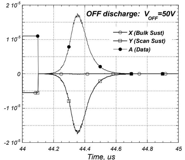
Figure 3. Current through electrodes during the select "OFF" discharge for the case of  $V_{OFF}=50\text{V}$ .
