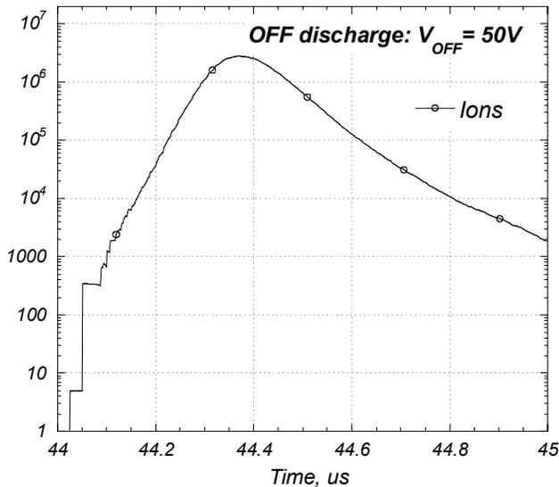
Figure 4. Number of ions in the gap during the "OFF" discharge for the case of  $V_{OFF}=50V$ .
