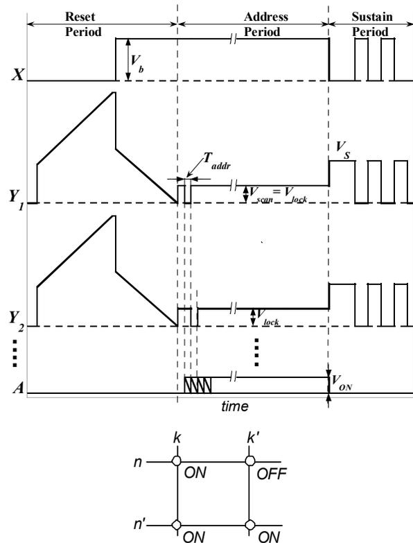
Figure 1. Conventional driving scheme. Three periods (reset/setup, address and sustain) are present. Locking the row after addressing prevents "OFF" cells ( $n, k'$ ) of the addressed row  $n$  from being ignited, when the cell ( $n', k'$ ) of the other row  $n'$  is being addressed "ON" later on.  $X$  and  $Y$  designate bulk and scan sustain electrodes, and  $A$  - the data electrode.
