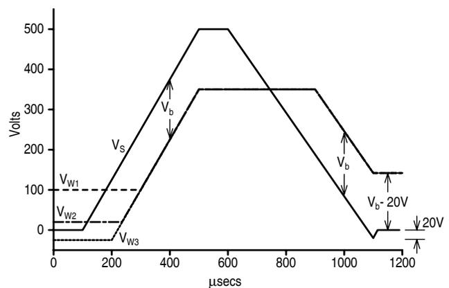
Figure 1. The applied voltage  $V_s$  and wall voltages  $V_w$  for three different initial wall voltages during the setup period. All end up with the same final wall voltage.
