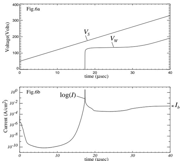
**Figure 6.** The voltages and current of a strong unstable discharge due to a too fast ramp rate, and insufficient priming.
