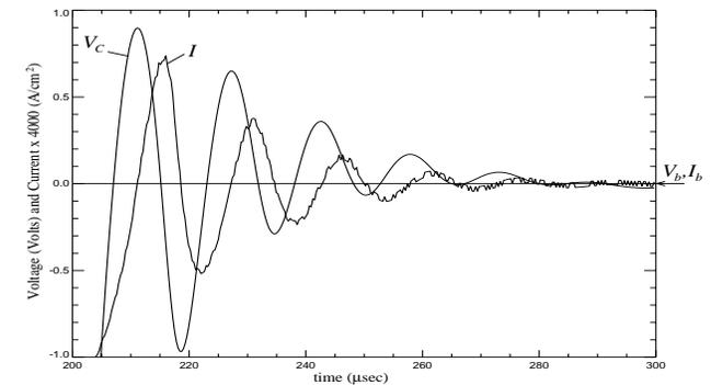
Figure 5. Expanded view of the voltage  $V_c$  and the current  $I$  of figure 4. These are expanded around  $V_b$  and  $I_b$ .
