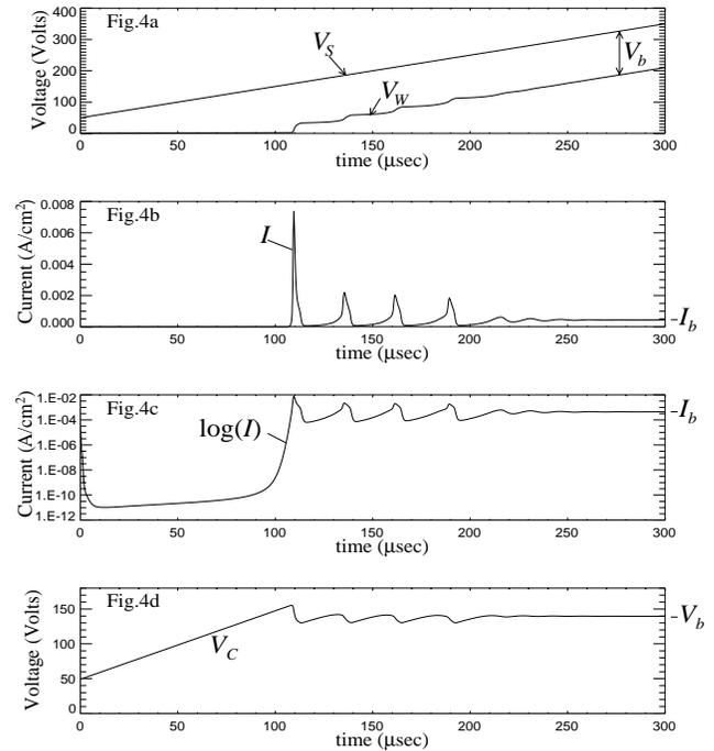
Figure 4. The voltages and currents that show the oscillations of the ramp discharge.
